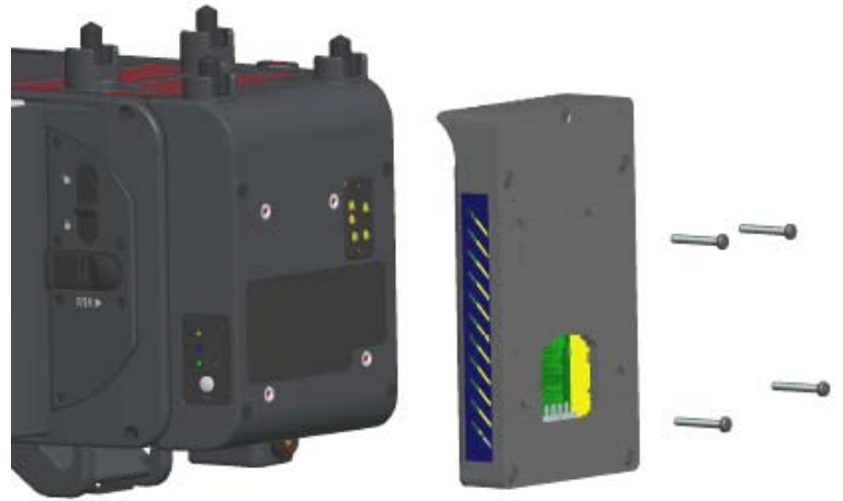
2. Fixing the adapter using 4 x 23mm screws
