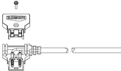
**Fig 3:** Remove the back half of the BSTAP housing. (Note: Be careful not to lose the spacer blank which seals the BSTAP side not being used).
