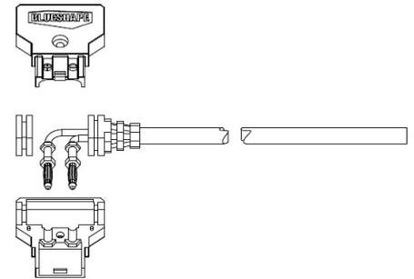
**Fig 4:** Place the Cable Strain Relief on the left side of the back half of the BSTAP Housing. Note: It is important that the banana pins fit properly into the slots of the BSTAP Housing.
